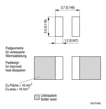
For superior solder joint connectivity results we recommend soldering under standard nitrogen atmosphere. Package not suitable for ultra sonic cleaning.
